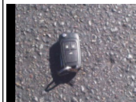
Same age asphalt surface following 3 applications of Enrichment treatment
